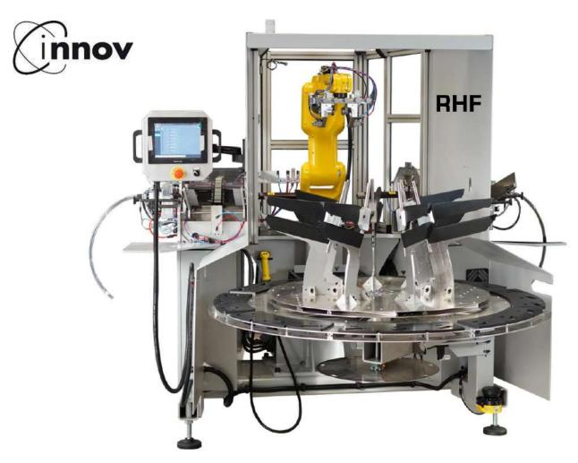
Thanks to its robotized arm, RHF is able to support almost any kind of hub and especially E-hubs. It is able to fill hubs that are even difficult to process manually as it can align flanges holes with spokes in a fast, precise and possibly complex movement.
